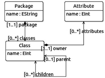
Fig. 7. Class diagram metamodel for model search.
