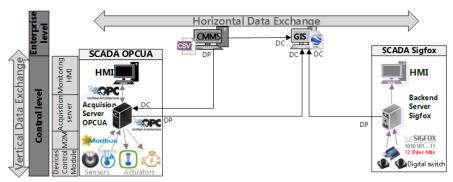
Fig. 1. Data Flow and exchange between heterogeneous systems
