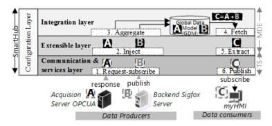
Fig. 4. Aggregating data from OPCUA server and backend server using smart-hub framework
