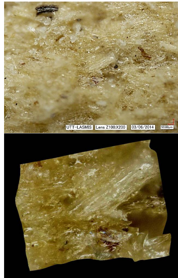
FIGURE 8. Starch matrix structure and 3D representation (50 \mu\text{m} scale X 200).
