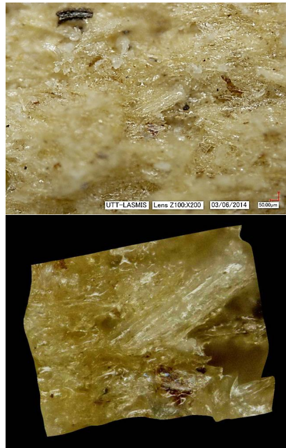
FIGURE 8. Starch matrix structure and 3D representation (50 μm scale X 200).
