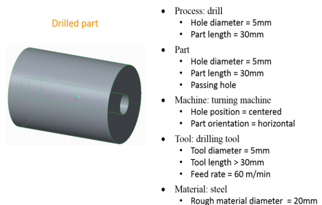
Figure 16 Final result for the drilled part
