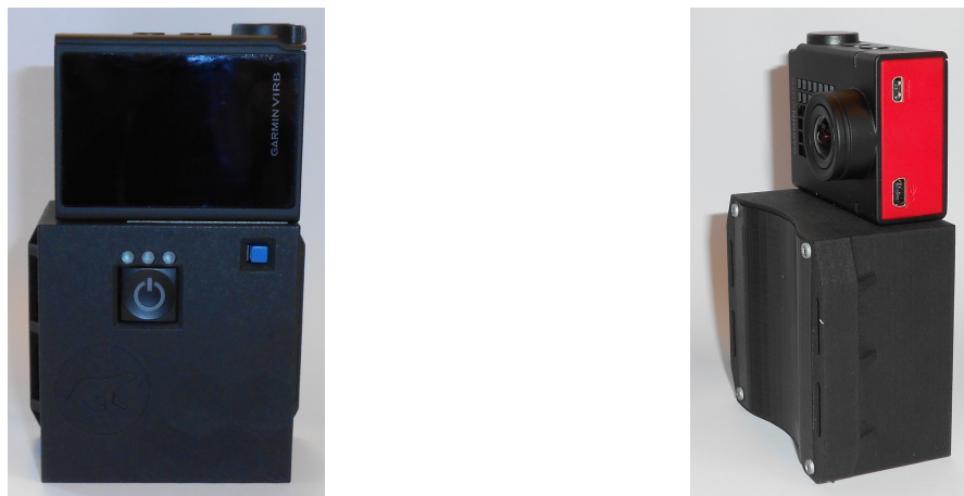
Figure 6. Hardware setup: the ULISS platform (below) and the Garmin VIRB camera (top).
