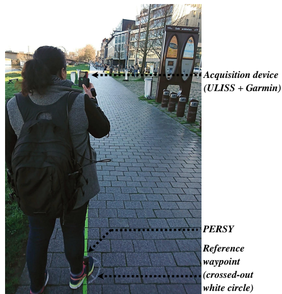
Figure 7. Handheld device (ULISS + Garmin), foot-mounted PERSY for reference track and reference waypoint.
