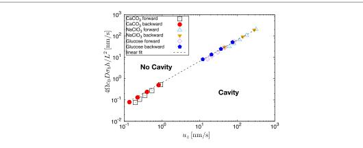
**Figure 3.** Non-equilibrium phase diagram for cavity formation for different materials and transition pathways. The scaled viscosity  $\bar{\eta}$  is assumed to be  $10^{-5}$  for CaCO<sub>3</sub> and  $10^{-2}$  for NaClO<sub>3</sub> and glucose.
