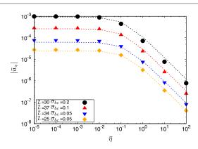
Figure B2. Growth rate  $|u_z|$  as a function of the viscosity shown in normalized units before undergoing the transition (flat growth) for different sizes. The dots are simulation results, the dashed lines were computed using (B.13) with L and  $\Delta \mu_b(\eta)$  (see (13)) measured in simulations and  $\Delta\mu_{eq}$  given by (B.5). The value of the contact size L varies weakly when the viscosity is varied.
