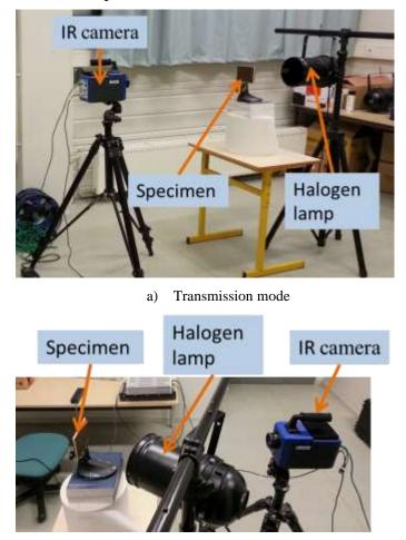
b) Reflection mode Figure 4. Infrared measurement
