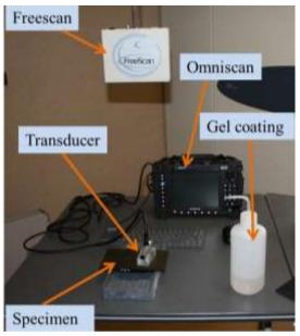
Figure 3. Ultrasonic measurement2.2.2Infrared Thermography
