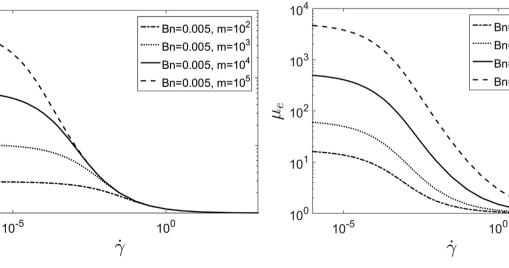
Fig. 1. Variations of viscosity  $\mu$  with  $\dot{\gamma}$  at the constant Bingham number (left) and constant regularization parameter (right).
