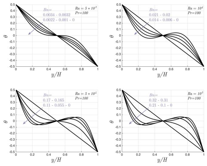
Fig. 8. Variations of non-dimensional Temperature  $\theta$  of Casson fluids for different Bn values along the vertical mid-plane for different values of Ra at Pr = 100.
