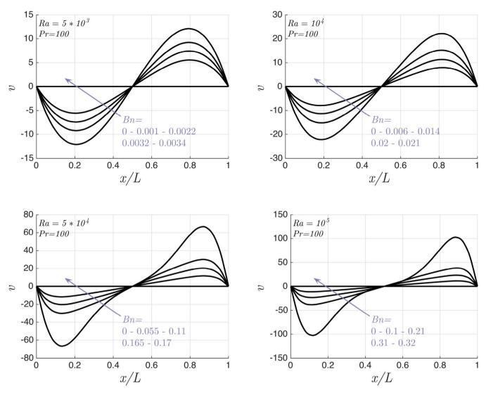
Fig. 7. Variations of non-dimensional velocity v of Casson fluids for different Bn values along the horizontal mid-plane for different values of Ra at Pr = 100.
