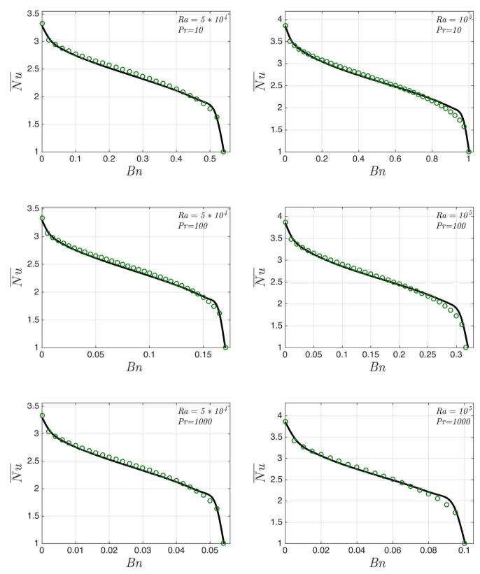
Fig. 11. Evolution of the mean Nusselt number of Casson fluids with the Bingham number for three different values of Pr at  $Ra = 5.10^4$  (left) and  $Ra = 10^5$  (right). [numerical results (-) and prediction of the correlation (o)given by Eq. (30)].
