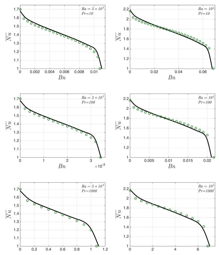
Fig. 10. Evolution of the mean Nusselt number of Casson fluids with the Bingham number for three different values of Pr at  $Ra = 5.10^3$  (left) and  $Ra = 10^4$  (right). [Numerical results (-) and prediction of the correlation (o)given by Eq. (30)].
