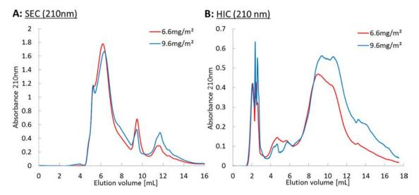
Figure 4. (A) Size-exclusion chromatograms and (B) hydrophobic interaction chromatograms of the adsorbed species as a function of the amount adsorbed at oil/water interfaces with UV detection at 210 nm (emulsions A and B from Table 1). Chromatograms were obtained by subtraction of the nonadsorbed species chromatograms from the total gum arabic chromatogram and rescaled to a concentration of 30 g·L<sup>-1</sup> to compare the molecular mass composition for each adsorbed film.
