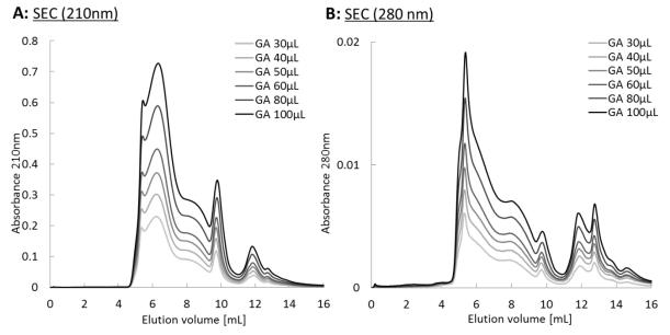
Figure S2: Size exclusion chromatogram of gum Arabic at 30g/L by varying the injected volume. (A) UV detection at 210nm, (B) UV detection at 280nm.
