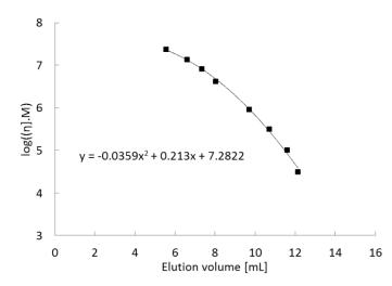
Figure S6: Universal calibration curve (realized with branched dextran of known molecular weight) for size exclusion separation on Biosuite 450Å SEC column (waters) with a flow rate of 0.8mL/min and 0.5M NaCl as the eluant solution.
