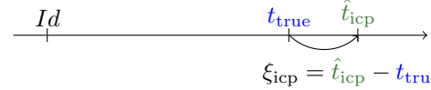
Fig. 2. Schematic illustration of the ICP procedure, error definitions and linearizations in the case of 1D translation t \in \mathbb{R} ( Id = 0 ).
