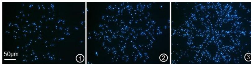
Figure S8. Pattern particle density as a function of the static contact time t_{sc} before the 500 nm latex dispersion drop dragging and fluorescent optical microscopy images of numbered assemblies.
