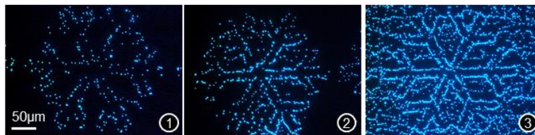
Figure S7. 1 \mu\text{m} latex particle pattern and background densities as a function of the stage temperature and fluorescent optical microscopy images of numbered assemblies.
