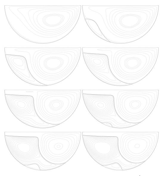
FIGURE 2. Streamlines of the steady state solution for  $\nu^{-1} = 500, 1000, 2000, 3000, 4000, 5000, 6000 \text{ and } \nu^{-1} = 7000.$
