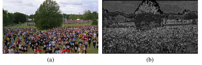
Fig. 2: (a) For crowdrun video sequence, Absolute difference (original-HVSP) for pre-processed frame(exaggerated by 100 times).
