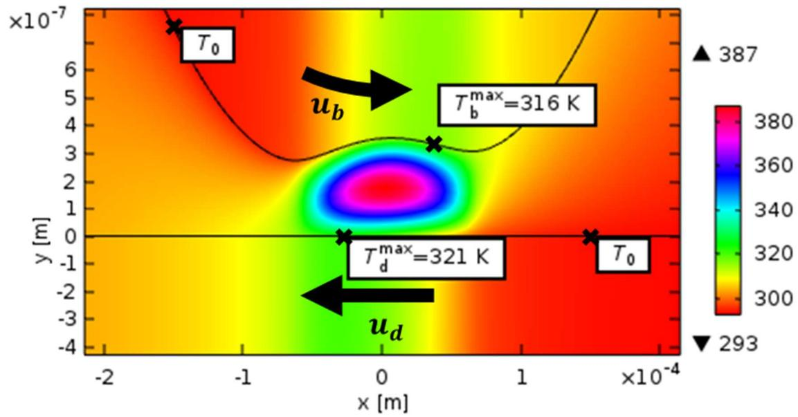
Figure 5 – Temperature variation in the fluid and solids for the reference case ( $u = 5 \text{ m/s}$ ,  $w^{1D} = 5.82 \times 10^4 \text{ N} \cdot \text{m}^{-1}$  and  $T_0 = 293.15 \text{ K}$ ). The equivalent body displacement is assigned to the top solid (steel). The bottom solid (sapphire) is considered rigid.
