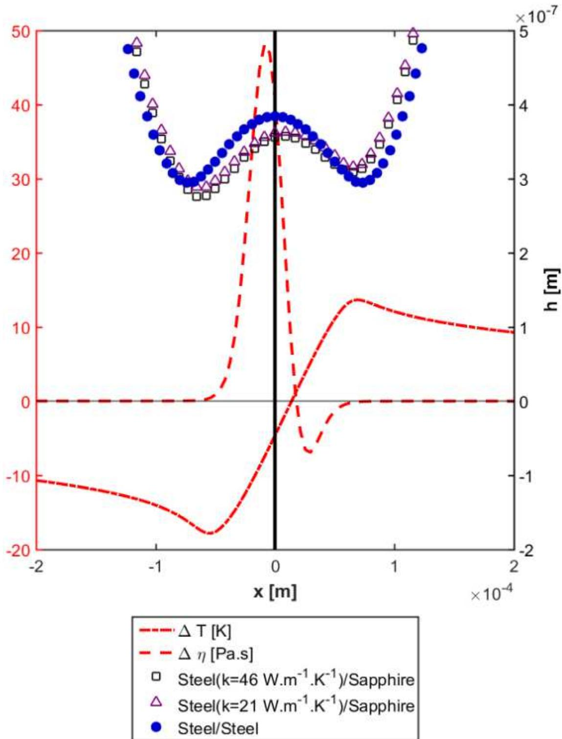
Figure 4 – For the reference case ( $u = 5 \text{ m/s}$ ,  $w^{1D} = 5.82 \times 10^4 \text{ N.m}^{-1}$  and  $T_0 = 293.15 \text{ K}$ ): On the left axis, temperature and viscosity differences between the fluid/steel interface and the fluid/sapphire interface for the steel/sapphire contact. On the right axis, numerical film thickness in the steel/sapphire contacts (two different values of  $k$ ) and the steel/steel contact.
