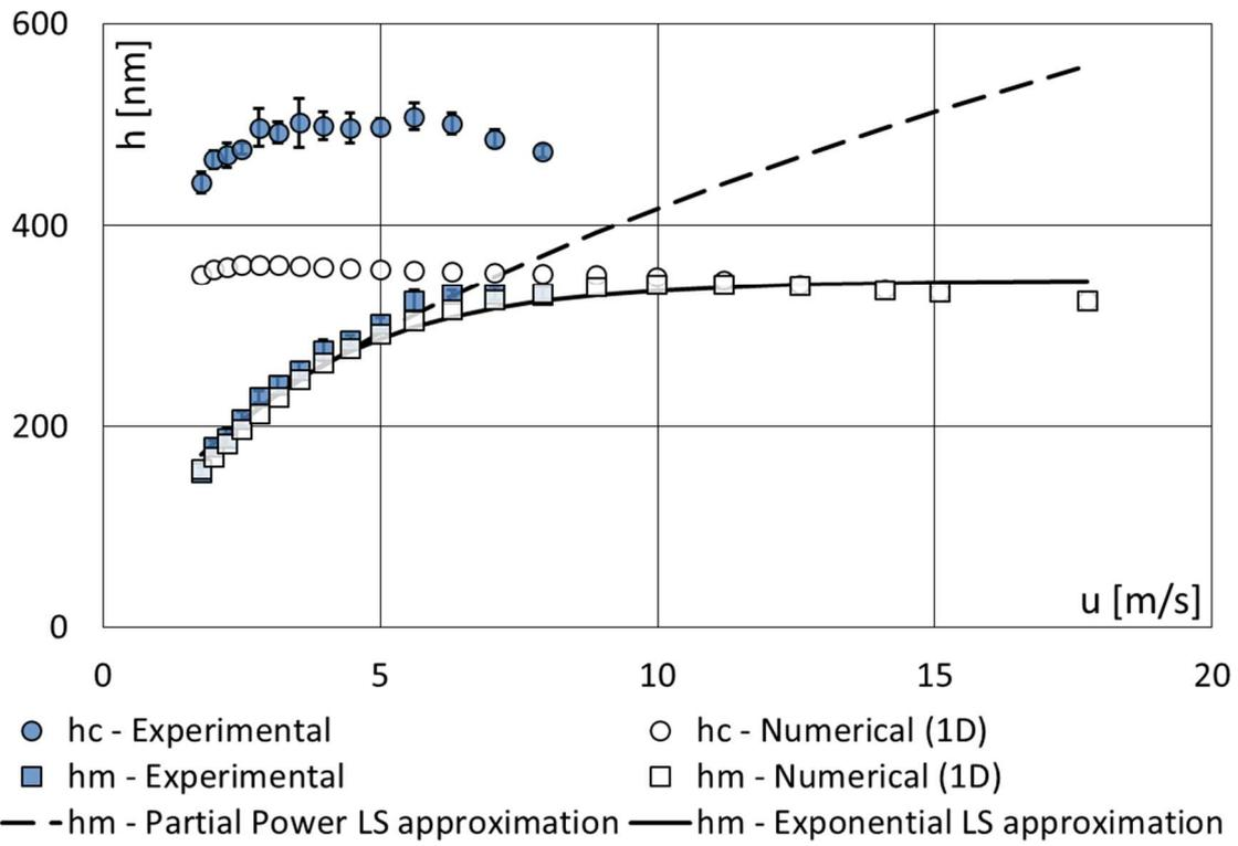
Figure 6 – Central and minimum film thickness variation with the surface velocity at  $w^{1D} = 5.82 \times 10^4 \text{ N} \cdot \text{m}^{-1}$  and  $T_0 = 293.15 \text{ K}$ .
