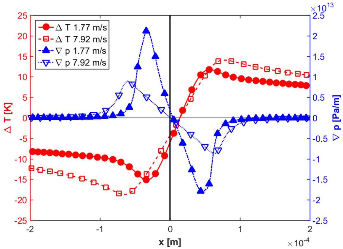
Figure 7 – Temperature differences (in red, left axis) between the two interfaces and pressure gradient (in blue, right axis) in the fluid at  $w^{1D} = 5.82 \times 10^4 \text{ N.m}^{-1}$  and  $T_0 = 293.15 \text{ K}$ , for two different surface velocities.
