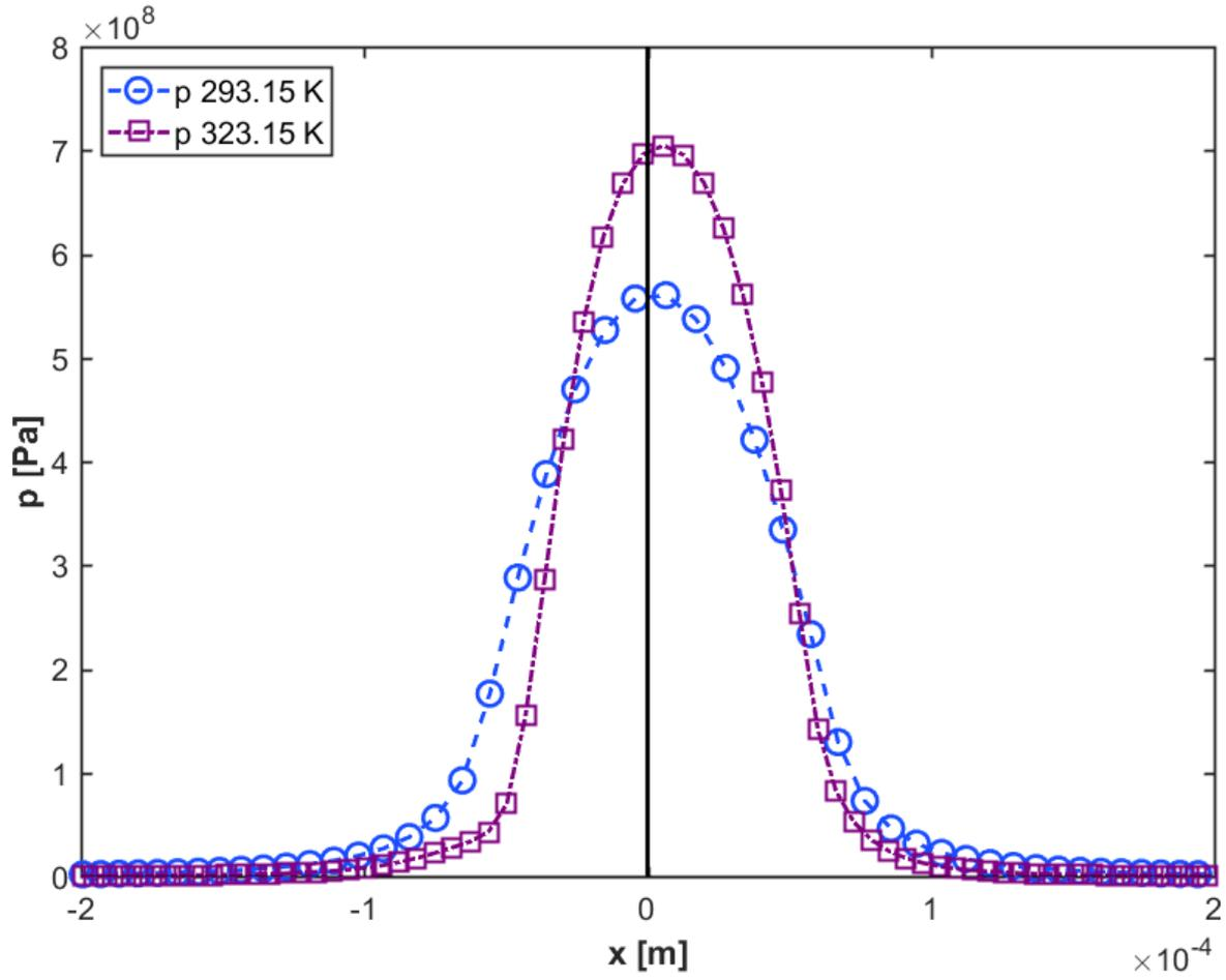
Figure 12 – Pressure profiles at  $u = 5$  m/s and  $w^{1D} = 5.82 \times 10^4$  N.m<sup>-1</sup>, for two different external temperatures.
