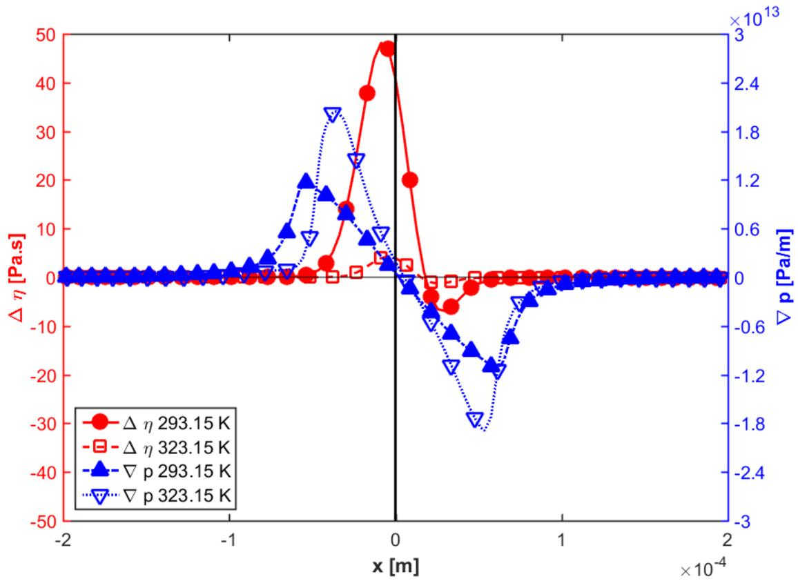
Figure 11 – Viscosity differences (in red, left axis) between the two interfaces and pressure gradient (in blue, right axis) in the fluid at  $u = 5 \text{ m/s}$  and  $w^{1D} = 5.82 \times 10^4 \text{ N} \cdot \text{m}^{-1}$ , for two different external temperatures.
