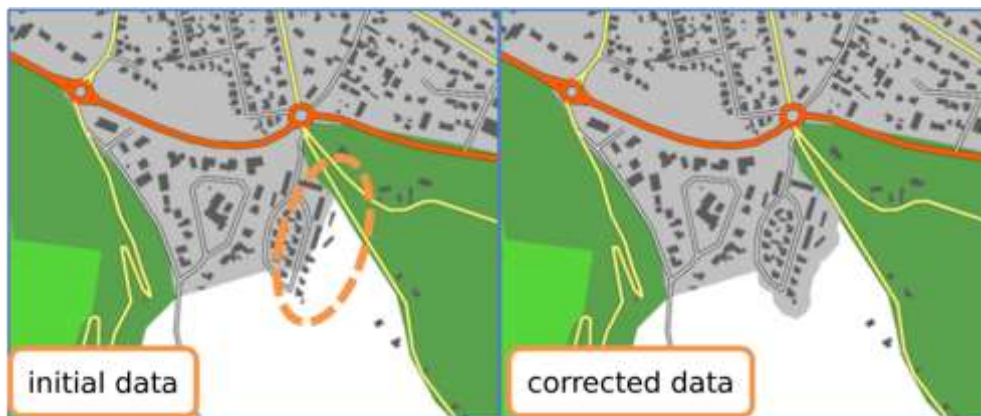
Figure 13. Initial data (©OpenStreetMap) with several buildings outside a low LoD built-up area. The correction (automatically obtained) increases the built-up area LoD and includes the inconsistent buildings in it.
