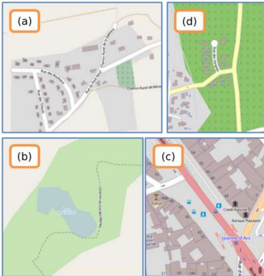
Figure 9. (a) building should be inside built-up area. (b) no intersection between paths and lakes. (c) bus stop should be along the road. (d) a group of houses should be in a clearing ©OpenStreetMap.
