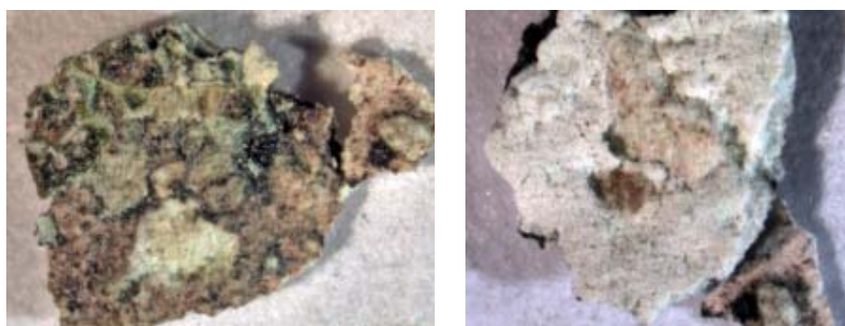
Images of P-124 sample surface and bottom where different layers could be observed.
