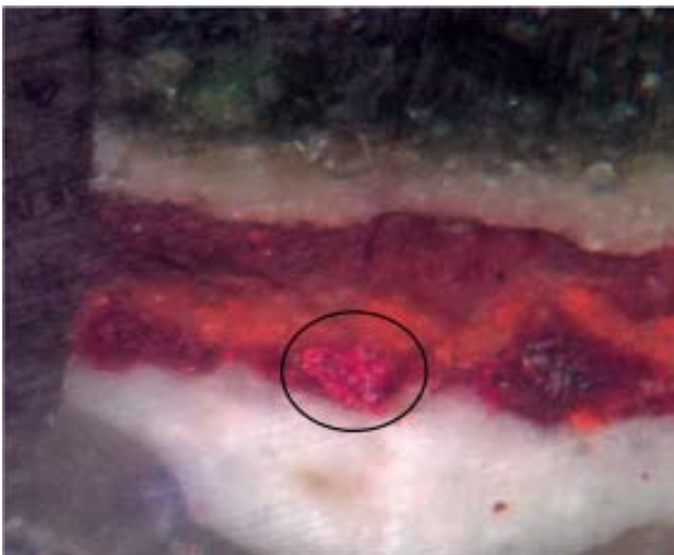
Optical microscopy image of the P-102 sample stratigraphy . On the bottom there is a white layer, and above that a red one where a grain of vermilion (black circle) appears.
