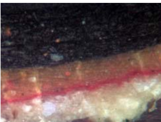
Image of optical microscopy of P-101 sample where the white layer could be seen.
