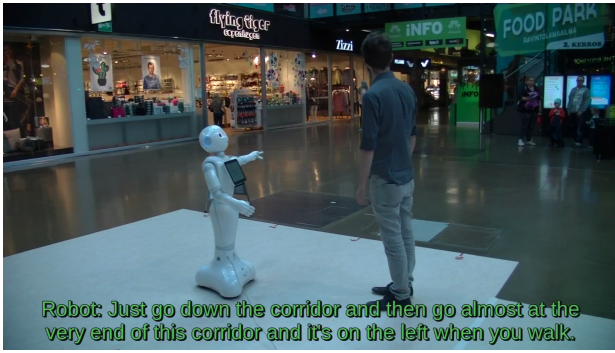
Fig. 10: Robot describing a route to a human in a mall using algorithms based on Ontologenus. The sentence in green is the explanation of the route verbalized by the robot and generated using the semantic representation stored in Ontologenus: "just go down the corridor and then go almost at the very end of this corridor and it's on the left when you walk".
