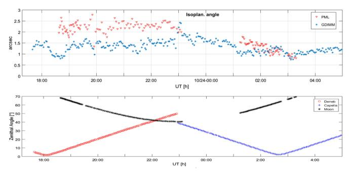
Figure 4. Top: comparison of isoplanatic angle deduced from PML  $C_n^2$  profiles and GDIMM scintillation measurements for the night of 2018 October 23. Bottom: zenithal angle of the Moon during the PML observations and of the stars observed by the GDIMM instrument.
