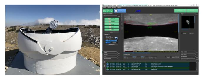
Figure 2. Left: the PML instrument inside its 12 ft AllSky dome. Right: the graphical user interface of the PML instrument showing the two Moon limb images.
