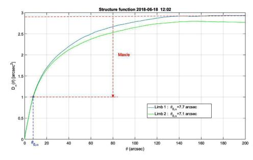
Figure 1. Example of AA fluctuation structure function obtained with the PML instrument on the Sun edge at the Calern Observatory on 2018 June 18.
