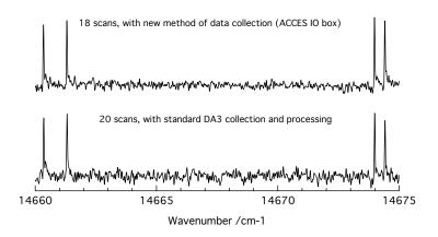
Figure 3: Spectra of <sup>60</sup>NiD collected and processed with the Bomem PCDA system (bottom, 20 scans coadded) and with the ACCES IO box and our own software (top, 18 scans). The signal-to-noise ratio in the bottom trace is about twice that of the top trace for a comparable number of scans.
