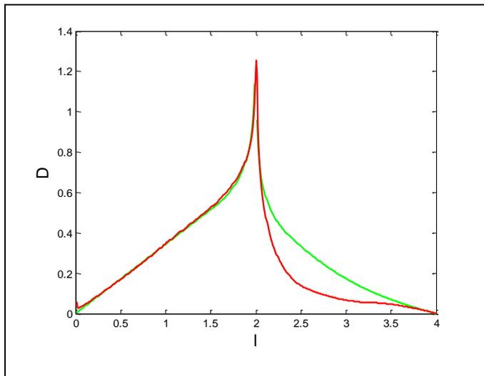
Figure 1: CLD for a capsule (hemisphere radius = 1, cylinder length = 2). red: MCS; green: our method.
