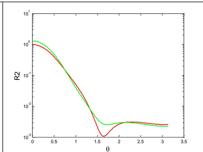
Figure 2:  $\langle |R|^2 \rangle$  as a function of the scattering angle (rad) for a capsule ( $R = 0.2\mu\text{m}$ ,  $H = 0.4\mu\text{m}$ ). red:  $D_l(l)$  from MCS; green:  $D_l(l)$  from our method.  $\lambda=450\text{nm}$ .
