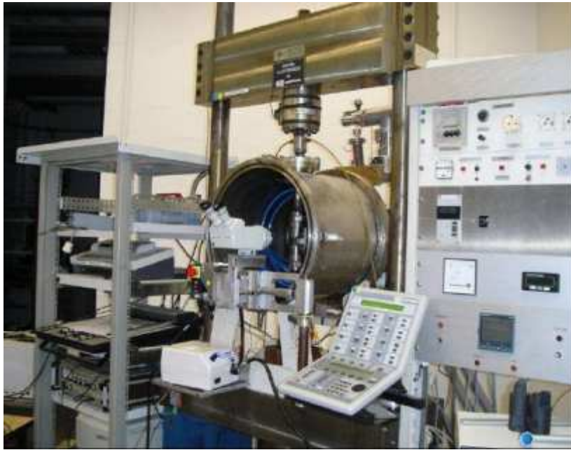
Figure 1. Fatigue crack growth test machine
