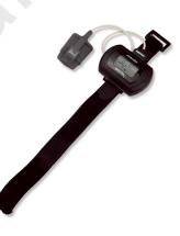
Figure 2: WristOx2 pulse oximeter
