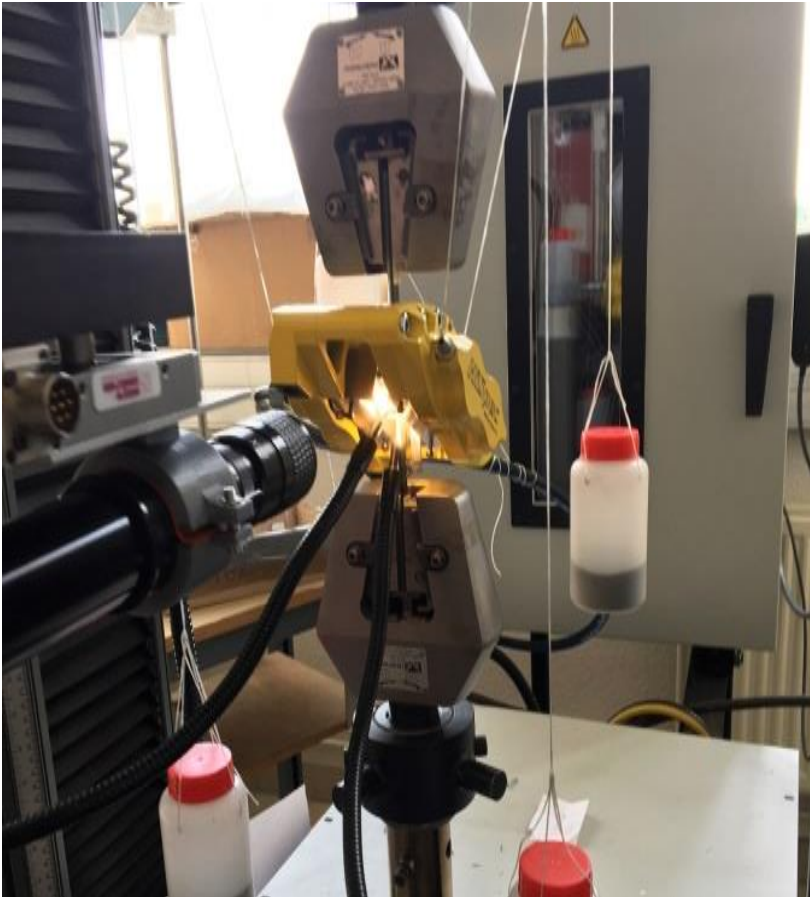
Figure 3: The compression system mounted on a tensile machine. The inclination of the caliper allows direct camera observation of the compressed specimen section.
