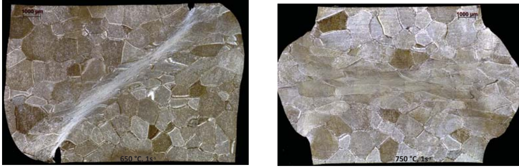
FIGURE 4: Metallographic observations of Ti17 specimens after deformation at a strain rate of 1 \text{ s}^{-1} for different temperatures.
