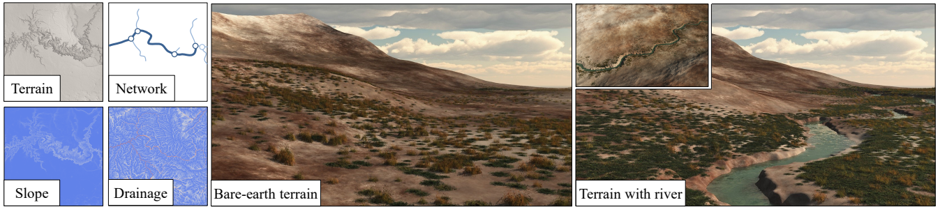
Figure 1: From a bare-earth input terrain, our method calculates the slope and drainage area to automatically generate a river graph that is procedurally amplified into a detailed river course. In this case, 4.266km-long, with 63k terrain and 42k flow primitives.
