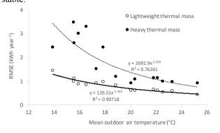
**Fig. 3.** *RMSE* of the metamodel for cooling energy needs versus the mean outdoor air temperature for the fifteen European climates.
