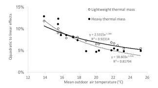
**Fig. 4.** Ratio of the quadratic to the linear effects versus mean outdoor air temperature for the fifteen European climates.
