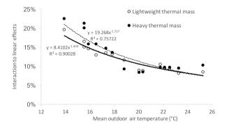
**Fig. 5.** Ratio of the interaction to the linear effects versus the mean outdoor air temperature for the fifteen European climates.
