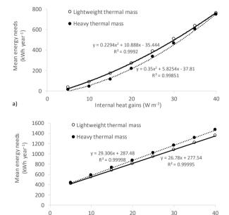
**Fig. 6.** Mean cooling energy needs as given by dynamic simulation versus internal heat gains: a) Helsinki and b) Athens.
