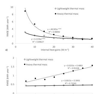
**Fig. 7.** *RMSE* of the metamodel for cooling energy needs versus internal heat gains: a) Helsinki and b) Athens.
