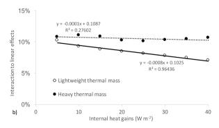
Fig. 9. Ratio of the interaction to the linear effects versus internal heat gains: a) Helsinki and b) Athens.
