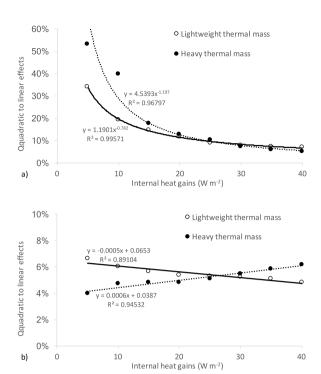
**Fig. 8.** Ratio of the quadratic to the linear effects versus internal heat gains: a) Helsinki and b) Athens.
