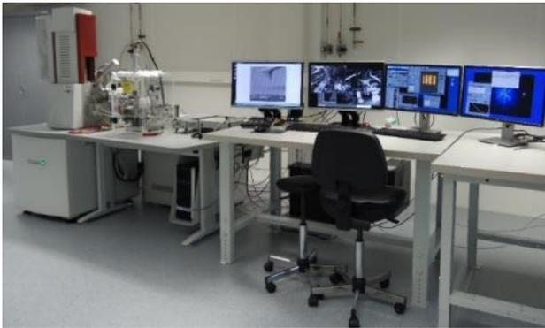
Fig. 6. Millimeter-wave NSMM integrated into a SEM.
