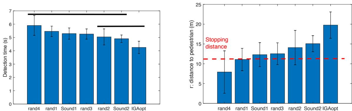
Figure 6. Bar graph of the average value of the *Detection time* (left) and *distance to pedestrian* (right) for the different EV sounds. Non significant differences between pairs of sounds ( $p > .05$ ) are linked with an horizontal line (paired t-test).
