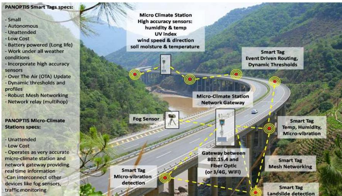
Figure 1 Topology of Network Smart Tags, Micro-climate stations and connected components in RI hot-spot
