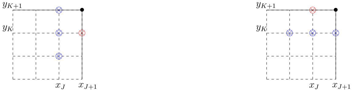
Figure 9: The stencil of the numerical boundary conditions (52b) and (54b) near the upper right corner. Left: the points (in blue crosses) involved in the computation of u_{J+1,K}^{n+2} (in red). Right: the points (in blue crosses) involved in the computation of u_{J,K+1}^{n+2} (in red).
