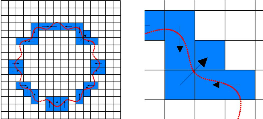
Figure 4: Flower-like interface ( $h = 1/16$ ). The interface is represented by red squares. Agglomerated cells are highlighted in blue. The arrows indicate how the agglomerations have been performed. Left: global view. Right: zoom near the cell where a diagonal agglomeration has occurred.
