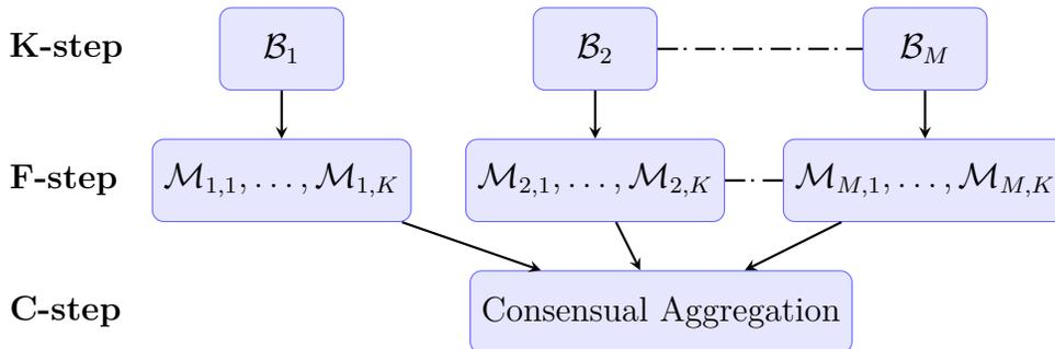
Figure 2: The main steps of the model construction: for each Bregman divergence  $\mathcal{B}_m$ , one model  $\mathcal{M}_{m,k}$  is fit per cluster  $k$ , then the models corresponding to the different divergences are combined.
