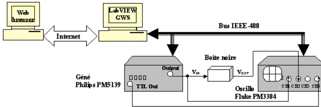
FIG. 3 – Application distante : banc de mesure gain-phase.
