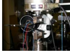
Figure 2. Mode I testing and opened sample.
