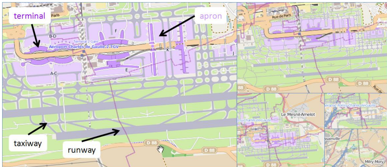
Figure 2. Highly detailed airport: when zooming out (pictures on the right), such details require generalisation. ©OpenStreetMap
