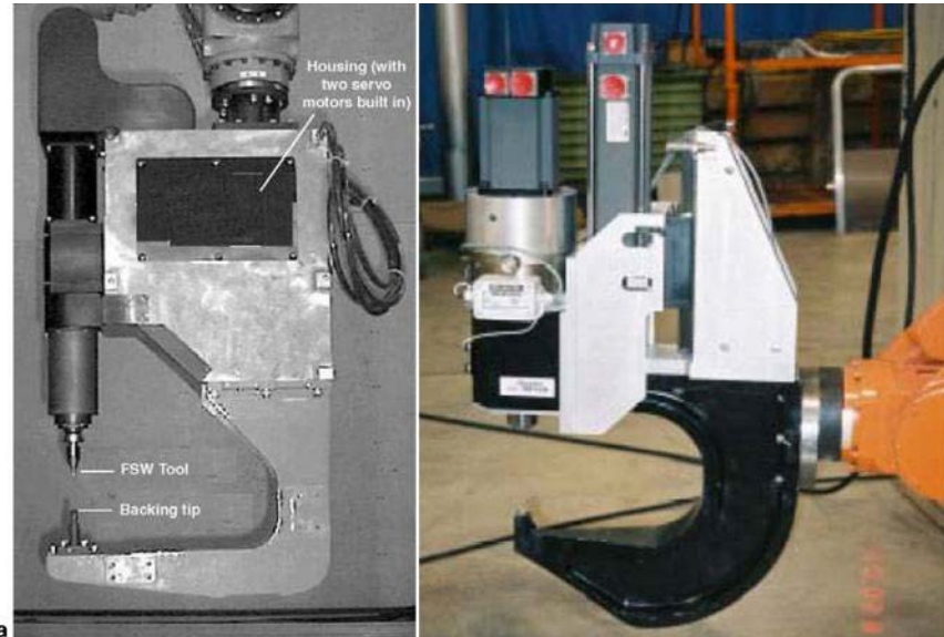
a spot FSW gun design; 1 b robotic FSSW 10 1 C frame device or spot FSW gun
