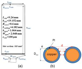
Fig. 4: (a) Slot dimensions (b) enamel covered wire
