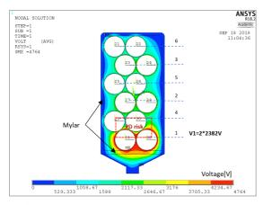
Fig. 10: Voltage map with  $V_1=2V_{cond1}$ ,  $e_{my}=480\mu m$  and  $e=85.5\mu m$
