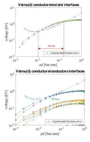
Fig. 8: Step 1 - *V<sub>simu</sub>*(*pd=d*) curves vs experimental Paschen curve (*e* max grade 3 [12])
