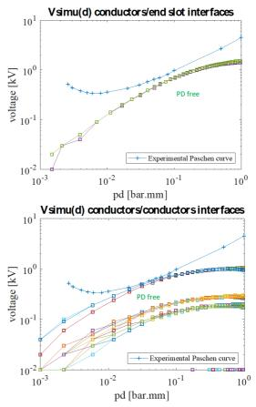
Fig. 9: Step 2 - V<sub>simu</sub>(pd=d) curves vs experimental Paschen curve (e<sub>my</sub>=480µm [11])
