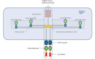
Fig. 1: Propulsion Chain of a Hybrid Aircraft [3]
