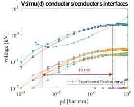
Fig. 11:  $V_{simu}(pd=d)$  conductor/conductor interfaces for overshoot 100% (ie.  $V_1=2V_{cond1}$ )
