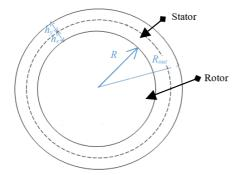
Fig. 2: Main sizes of electric motor
