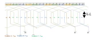
Fig. 3: Stator winding configuration: concentric winding with 6 conductors per slot.
