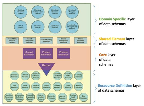
Figure 1: IFC layers of data schemas (ISO 16739-1) and modelled in the EXPRESS Schema (ISO 10303-11).
