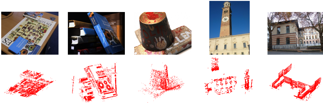
Figure 10: Sample images of five datasets and the reconstructed 3D point clouds. From left to right: poster (17 images), book (53 images), pot (21 images), tower (21 images) and CAB (300 images).
