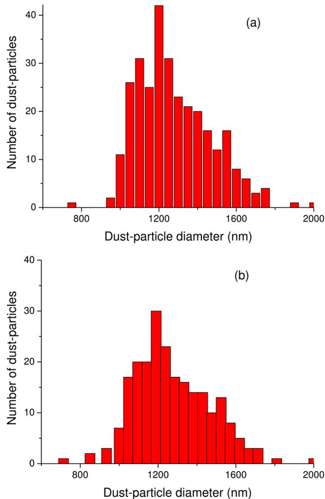
FIG. 6. Size distribution of collected spherical dust-particles in (a) clean and (b) coated conditions.
