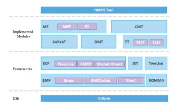
Fig. 8. HMCS tool architecture (collaboration concepts' are embolden).
