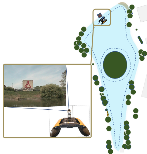
Figure 3. GTL's Clearpath Kingfisher collected the surveys of the Symphony Lake Dataset. It navigated the path shown as the dotted line with its camera facing towards the shoreline.
