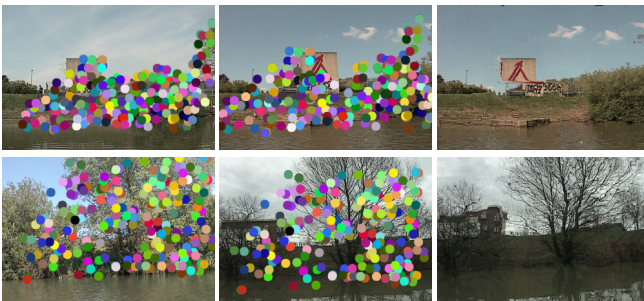
Figure 20. Noise in aligned images. (top) Map points from two surveys are projected onto the reference image (left) and the image to be aligned (middle). Their inconsistency caused the error of the aligned image (right), which otherwise had a strong appearance-based correspondence. (bottom) The alignment process added noise to the tree structure in the well-aligned image (right), even though the map point priors were consistent.
