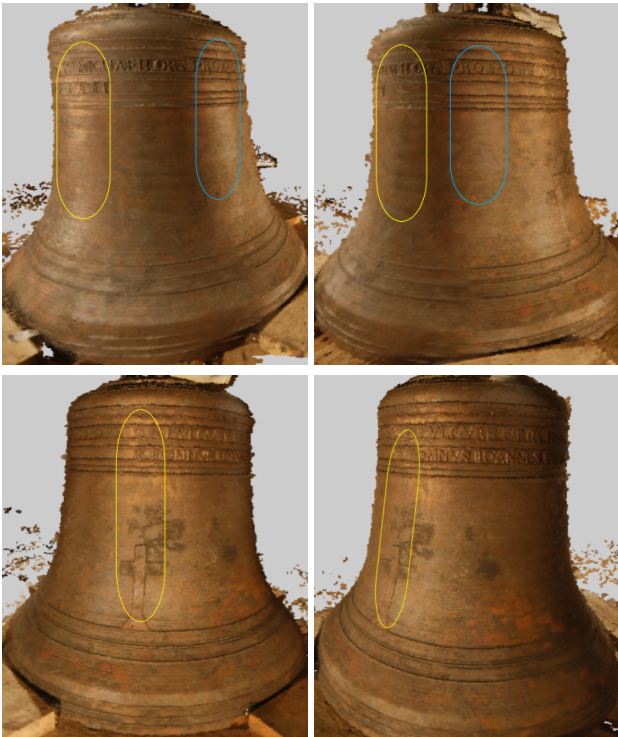
Fig. 9. View-dependent appearance: Highlights move according to the observer. Top: Two regions on the object are encircled, the highlight visible on the yellow and blue regions disappears on the right image (the text on the top of the bell can be used as reference). Bottom: The highlight in the yellow region moves on the right according to the viewpoint.
