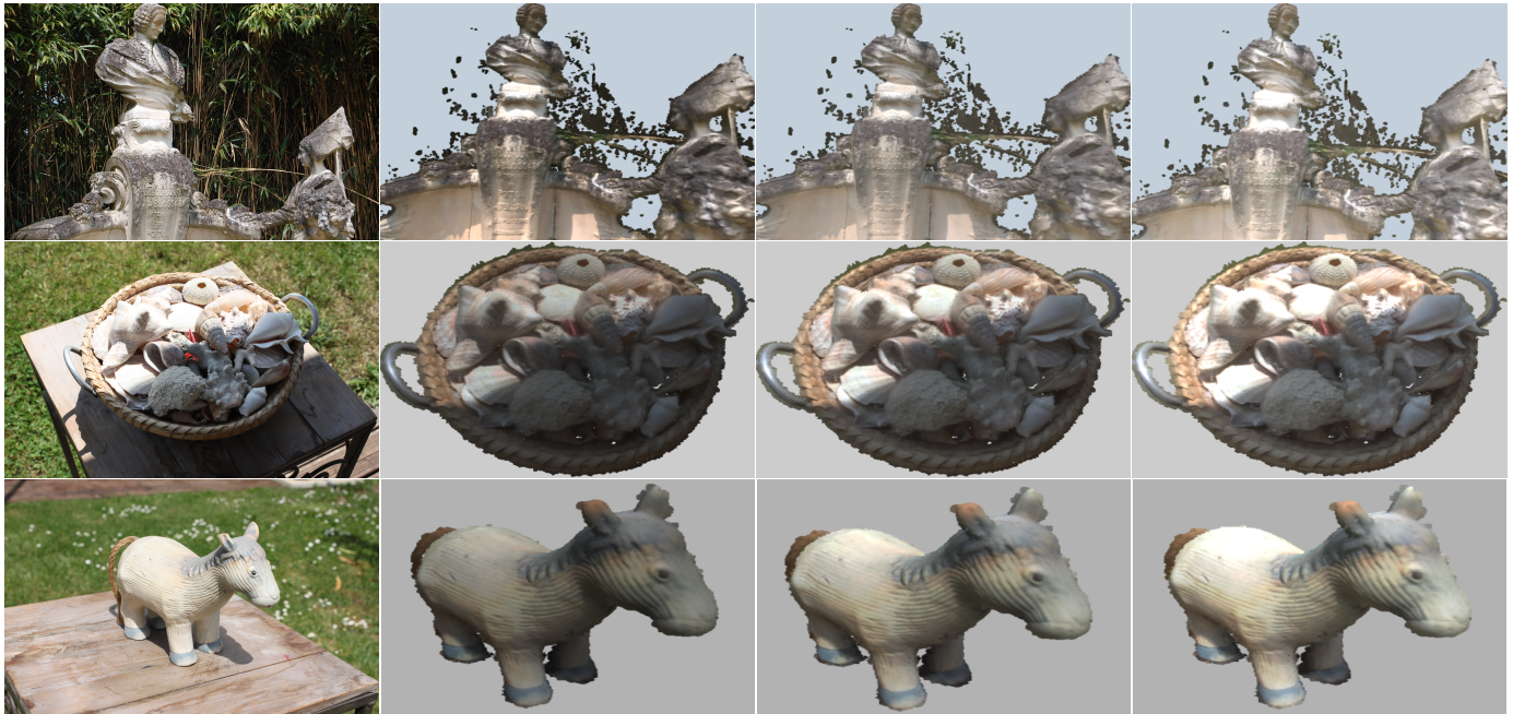
Fig. 11. Interactive HDR rendering with exposure control, with scenes captured from 3 or 4 different series of photographs. For each line: An original photograph and 3 different exposures rendered with our system. Statue (first line), Seashell (second line); Horse (third line).
