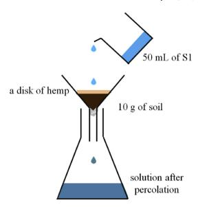
**Scheme 3.** Percolation procedure: this is an extraction process that involves the slow descent of solution S1 through the soil, in absence or presence of a hemp disk; the number of passes through the system was 1, 5, 10 or 15.
