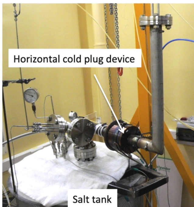
Fig. 3. Configuration of the first tests with a simple vertical pipe instead of the loop circuit.
