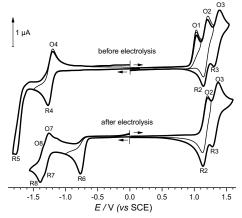
**Figure 4** Cyclic voltammetry of a  $10^3$  M solution of **1** in CH<sub>2</sub>Cl<sub>2</sub> 0.1 M TBAPF<sub>6</sub> before (top) and after (bottom) electrolysis at  $E_{\rm app}$  = 0.96 V/SCE (2.5 F),  $\nu$  = 100 mV.s<sup>-1</sup>, WE: Pt, Ø = 1 mm.
