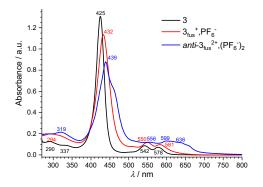
Figure 3 UV-vis. absorption spectra of 3,  $3_{fus}^+$ , $PF_6^-$  and  $anti-3_{fus}^2$ +, $(PF_6^-)_2$  in DMF ( $C = 7.5 \times 10^{-6}$  M, I = 1.00 cm).
