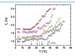
**Figure 2.** Free volume  $f_v$  (%) as a function of temperature assessed from PALS for ( $\square$ ) PLA 0%, (blue ring) PLA 2.5%, (green triangle) PLA 5%, (purple diamond) PLA 9%, and (brown star) 13% ATBC. Arrows correspond to the signature of the glass transition obtained from PALS.
