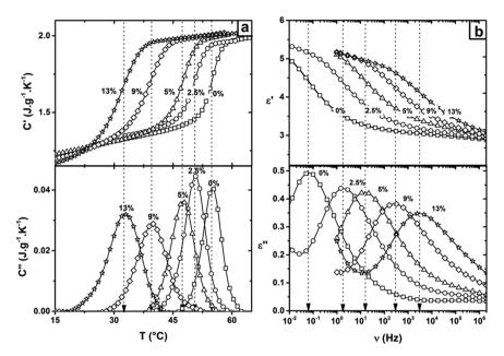
Figure 1. ( $\square$ ) PLA 0%, ( $\bigcirc$ ) PLA 2.5%, ( $\triangle$ ) PLA 5%, ( $\diamondsuit$ ) PLA 9%, and (star) ATBC 13%. (a) MT-DSC in-phase (C') and out-of-phase (C'') components of the complex heat capacity versus temperature. Arrows illustrate the MT-DSC midpoint of the glass transition (b) DRS real part ( $\varepsilon'$ ) and imaginary part ( $\varepsilon''$ ) of the complex permittivity versus frequency at 332 K. Arrows depict the maximum frequency of the main relaxation process.
